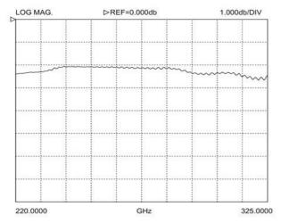
Typical insertion loss of a Model 325B-GSG-80-BT
