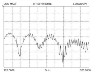
Typical uncalibrated performance of a Model 325B-GSG-80-BT while touching a 50 ohm load on our CS-15 calibration substrate.
